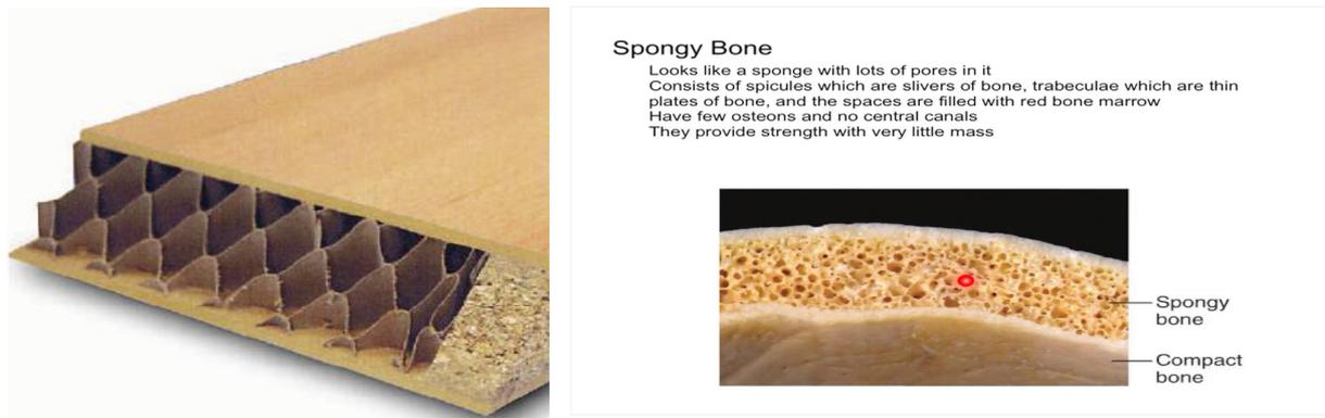
Comparison of an artificial (wood and paper) composite structural sandwich with a cross section of the parietal bone.
